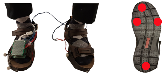
Figure 7: Shoe controller prototype and positions of foot pressure sensors (red dots).
